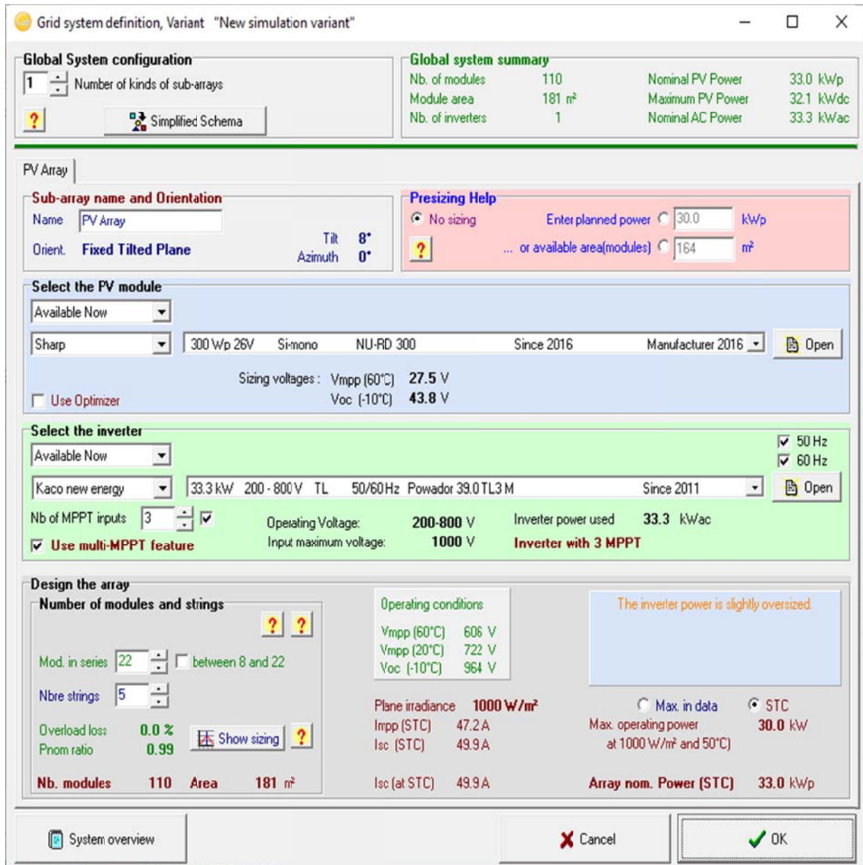
Figure 5 The system configuration used for the simulation of the grid-connected PV power supply system
