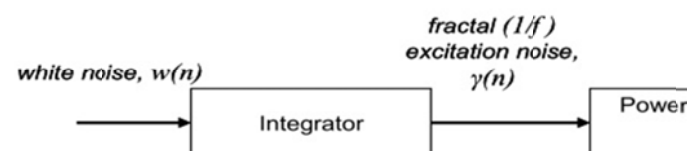
Fig. 1. Model for quasi-continuous modal disturbances in a power system
